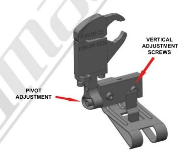
STEP 6 - Install your radar detector onto the mount. Use the adjustments shown above to adjust the RD to your desired position. We recommend adjusting the RD as close to the bottom of your mirror as you can. Be sure to tighten all adjustment screws after the adjustments are made.
