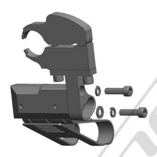
STEP 5 - Reinstall the BODY ASSEMBLY. Be sure to include the lock washer with the top socket head screw and the lock and flat washer with the bottom socket head screw as shown above. NOTE: there are extra lock and flat washers included in the tool kit just in case you happen to misplace one.
